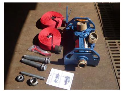
Figure 2-15. Simulated Runoff Test Equipment (PWD)
