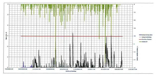
Figure 2-26. Rainfall (green) and water level response (black) time series in a biofiltration facility. The red line represents the overflow elevation. Three overflow events occurred in two years (Borough of Etna GROW project).
