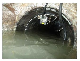
Figure 2-8. Area Velocity Meter Installation Setup in Sewer (RJN Group)
