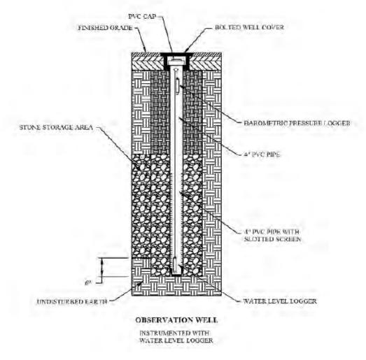
**Figure 2-17. Example Monitoring Well Schematic (PWD).** Includes Water Level and Barometric Pressure Sensors. Note the sump depth is 6".
