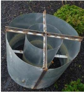
**Figure 2-23. GSI Infiltrometer Testing. (PWD)** Single Ring Infiltrometer Test on Permeable Pavement; Double Ring Infiltrometer Test on Bioretention Soils
