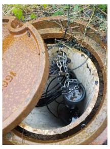
Figure 2-12. Pressure transducer installed in monitoring well (PWSA)
