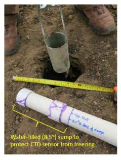
**Figure 2-24. Field measurement of sump depth** (East Liberty Presbyterian Church monitoring program [John Buck, CEC])
