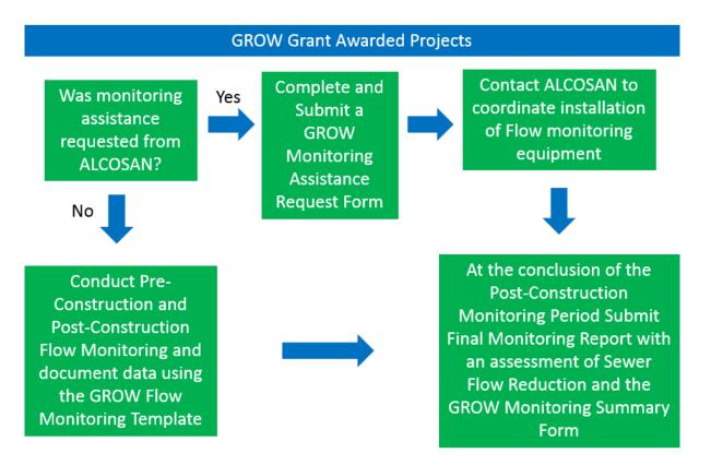
Figure 1-1. Monitoring Process Flowcharts for Pre- and Post-Construction Monitoring
