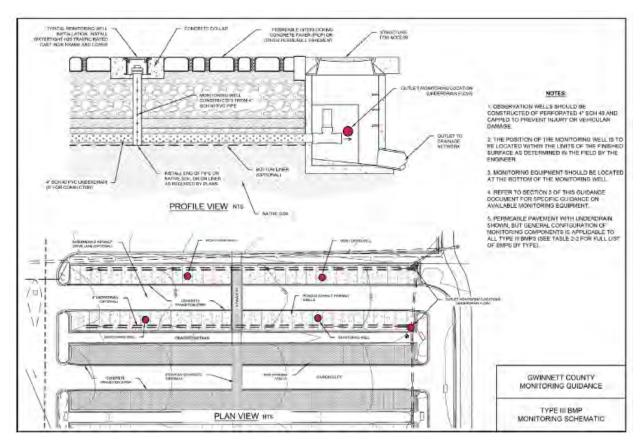
Figure 2-20. Example Schematic of a Permeable Pavement Site (Gwinnett County) In-GSI Monitoring Locations at the Outlet and Multiple Wells
