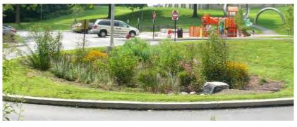
Figure 2-4. Bioretention in a Parking Lot Island
