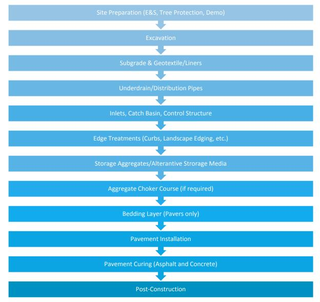
Figure 2-22 General Construction Sequence for Permeable Pavement Systems
