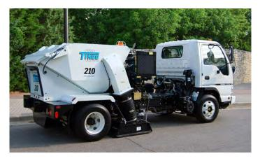
Figure 2-12. Vacuum Sweeper Regenerative air sweepers blow air on pavement surfaces to loosen dirt and debris during vacuuming.
