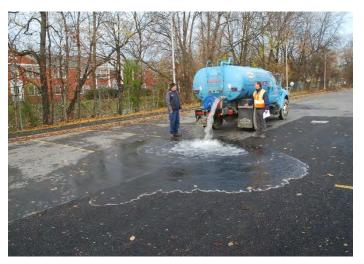
Figure 2-13. Permeable Pavement Testing
