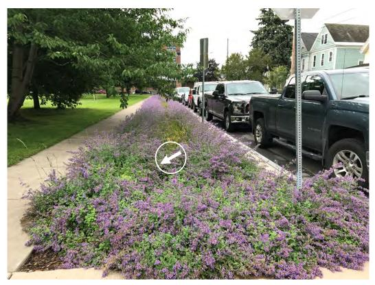
Figure 3-2. Bioswale in Highly-Visible Site
