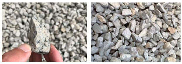
**Figure 2-9. Aggregate with Fines** *Example of unacceptable GSI facility aggregate*
