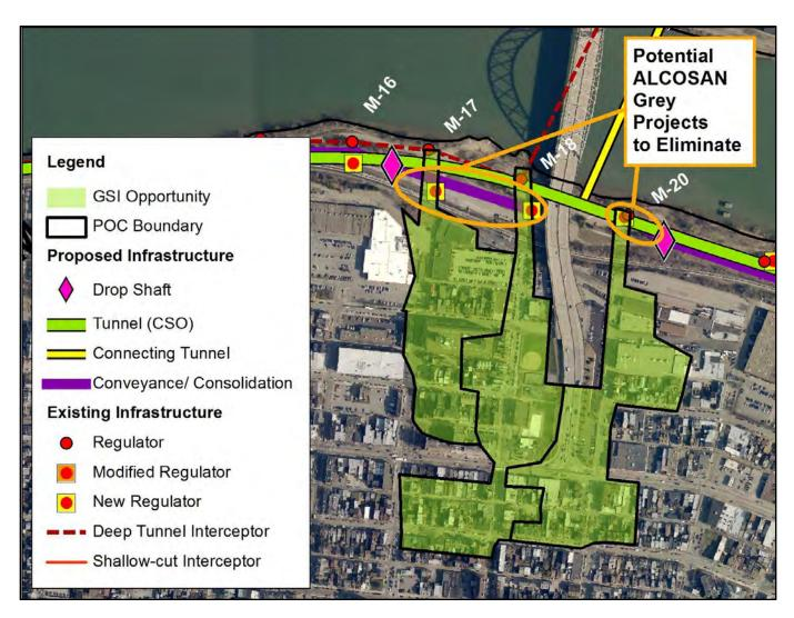
Figure 3-24: Example of Evaluating Opportunities to Eliminate Grey Projects with GSI for Outfalls M-17, M-18 and M-20
