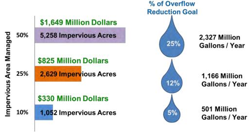
Figure 3-13: Capital Cost and Overflow Reduction Benefit of Green Stormwater Infrastructure (Simulations 1, 2, 3)
