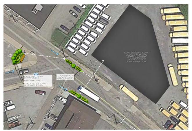
Figure 4-22: Etna Borough GSI Concept Plan
