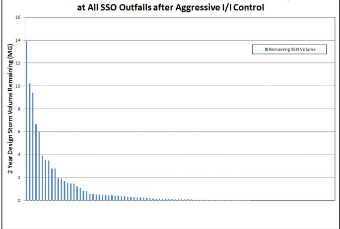
Figure 3-30: Remaining SSO Volume After Aggressive I/I Reduction
