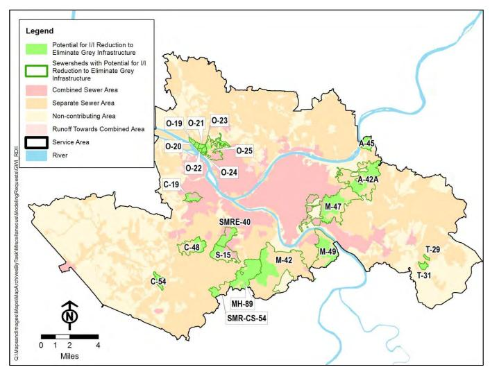
Figure 3-29: Location of Point of Connection Sewersheds with Greatest Potentials for I/I Reduction to Eliminate SSOs for 2-Year Design Storm
