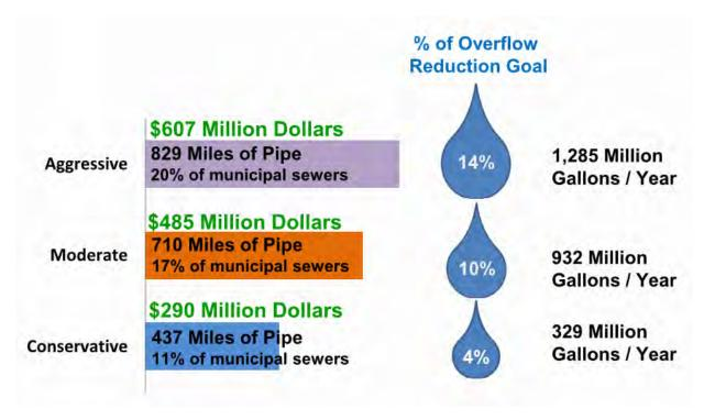
Figure 3-16: Capital Cost and Overflow Reduction Benefit of I/I Reduction (Simulations 4, 8, 9)
