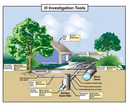
Figure 2-2: Pathways of Infiltration and Inflow (I/I) into Sanitary Sewer Systems and Various I/I Investigation Tools
