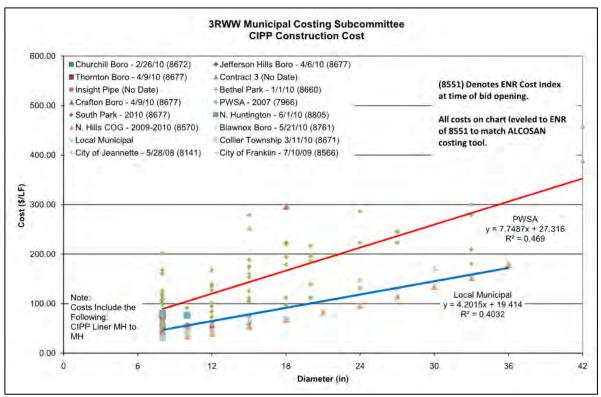
Figure 3-12: Data Plot of Local CIPP Construction Data
