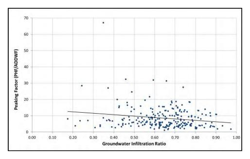
Figure 3-11: Relationship between Wet Weather Peaking Factor and Groundwater Infiltration in the ALCOSAN Service Area
