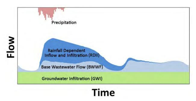
Figure 3-10: Three Components of Wastewater Flow in Separate Sanitary Sewer Systems
