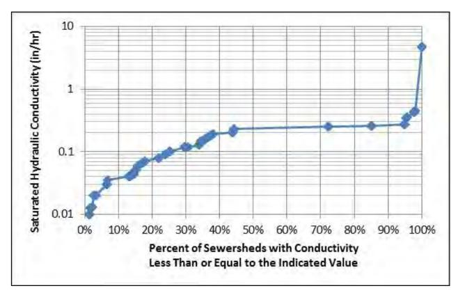
Figure 3-3: Cumulative Distribution of Saturated Vertical Hydraulic Conductivity
