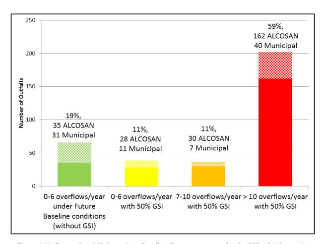
Figure 3-22: Count of outfalls in various Overflow Frequency ranges for the GSI only Alternative
