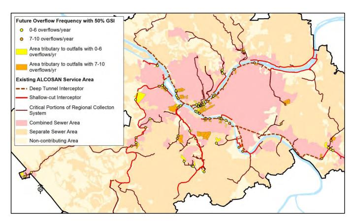
Figure 3-23: Outfalls in various Overflow Frequency ranges for the GSI only Alternative
