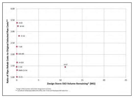
Figure 3-28: Potential of I/I Reduction to Eliminate SSOs – Point of Connection Sewersheds– Cost Ratio of One or More
