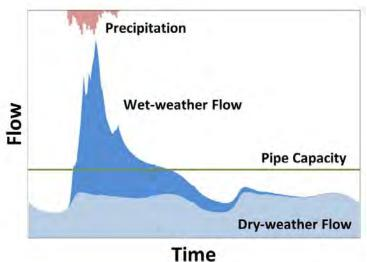
Figure 6-1: Controlling sewer overflows requires the capture and treatment of large amounts of wastewater which frequently exceeds current system capacities
