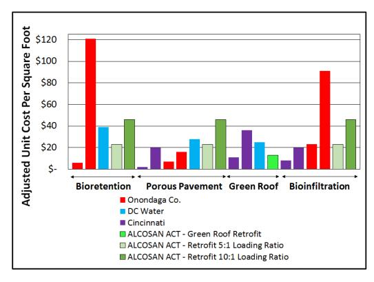
Figure 3-7: National Comparison - Construction Cost (\$ per Square Foot) of Installed GSI
