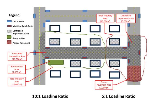
Figure 3-4: Illustration of Loading Ratio Definition
