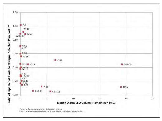
Figure 3-27: Potential of I/I Reduction to Eliminate SSOs – Point of Connection Sewersheds – Cost Ratio of One or Less
