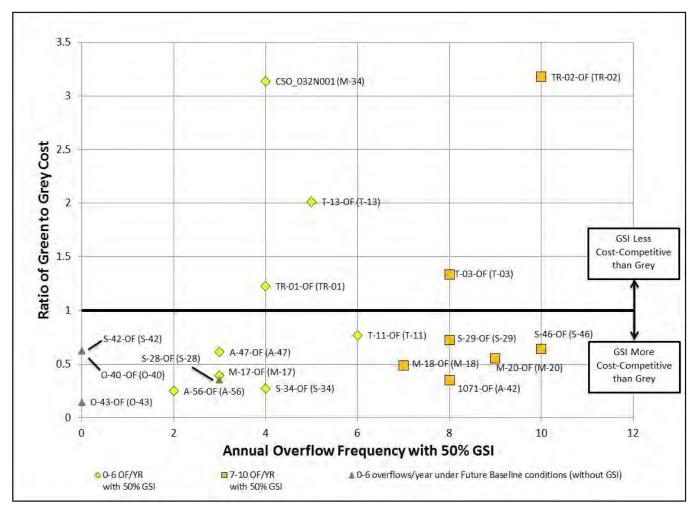
Figure 3-25: Cost Comparison Results for 19 Outfalls Analyzed with 50% of Impervious Cover Managed with GSI
