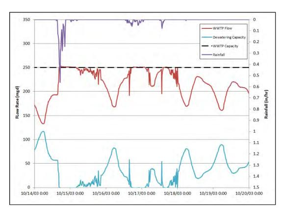
Figure 3-1: Example of System Wet Weather Treatment and Dewatering Capacity
