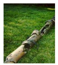
Figure 6-4: Deteriorated Building Lateral Sewer
