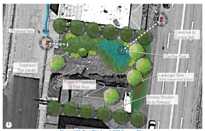
Figure 4-25: East Pittsburgh GSI Concept Plan
