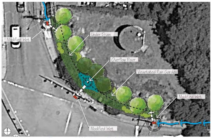
Figure 4-26: ALCOSAN Access Shaft M-30 GSI Concept Plan
