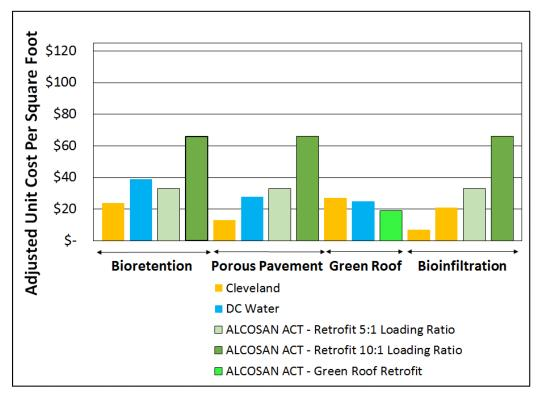
Figure 3-8: National Comparison - Capital Cost (\$ per Square Foot) of Installed GSI
