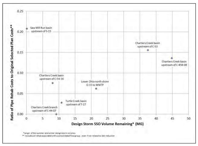
Figure 3-26: Potential of I/I Reduction to Eliminate SSOs - Groups of Points of Connections
