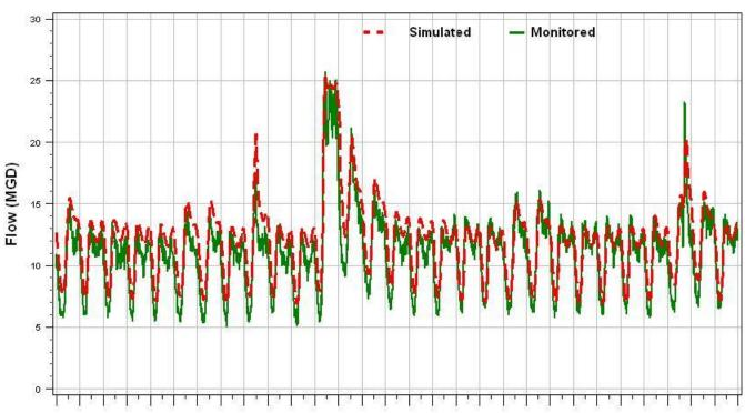
Figure 4-16: Typical Example of an H&H Model Validation Plot Comparing Simulated and Observed Wastewater Flow
