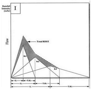
Figure 4-12: Three triangular unit hydrographs used in the H&H models to represent the sewer system response to a storm event
