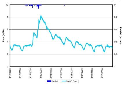
Figure 4-11: Example of a monitored sewer system response to a storm event showing typical storm peak and recession limb
