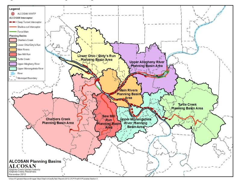
Figure 3-6: ALCOSAN Planning Basin Configuration
