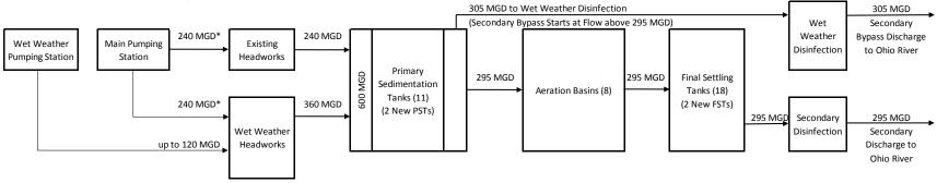
INTERIM MEASURES WET WEATHER PLAN (600 MGD FLOW CONDITION SHOWN)
