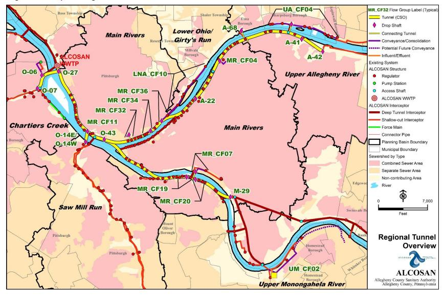
Figure 11-4: Proposed Regional Tunnel Extent for Interim Measures Wet Weather Plan
