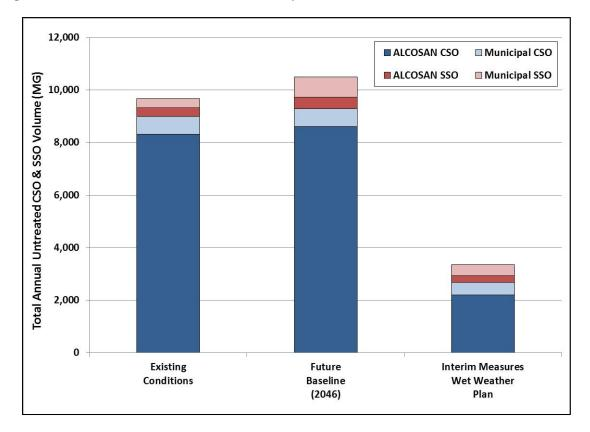
Figure 11-9: Overflow Volume Reduction Comparison for Interim Measures Wet Weather Plan
