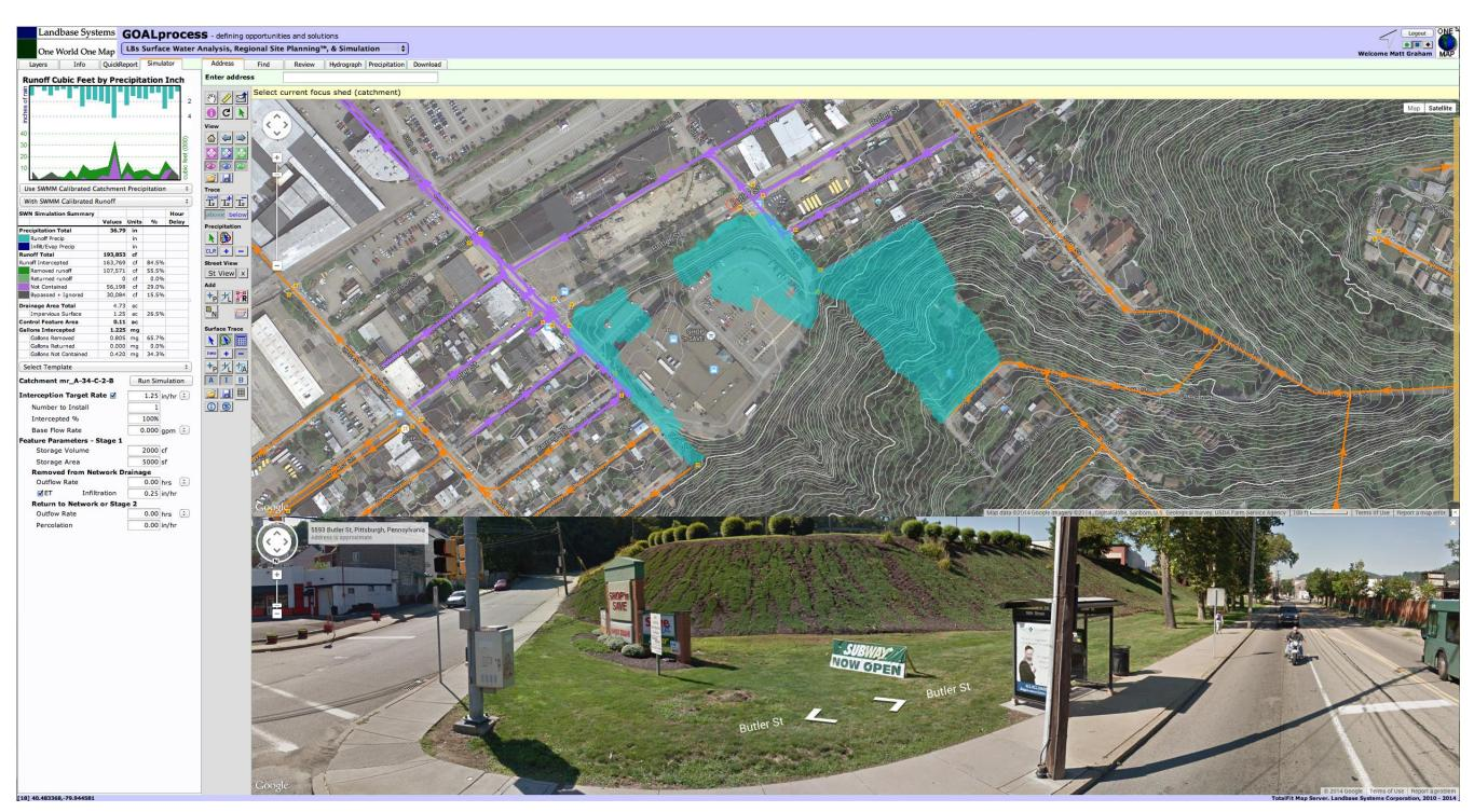
Multiple known upstream inlets exist within/adjacent to the current defined gross drainage area. Also, three to five private inlets could be added to the gross drainage of this GSI feature.
