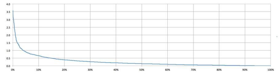
The top 12.6% highest net runoff ranked inlet locations appear to receive 50% of runoff tributary to known inlets in sheds A-22 through A-35.
