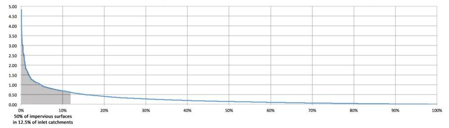
The top 12.5% highest 'net impervious' ranked inlet catchments contain 50% of tributary impervious acres in sheds A-22 through A-35.
