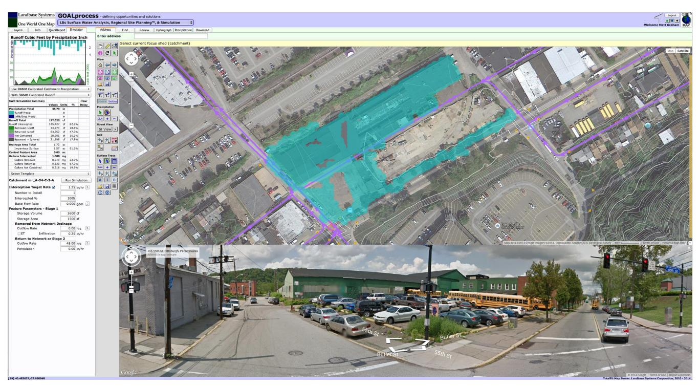
One known upstream inlet exists within the current defined drainage area. Rooftop drainage areas need to be verified.
