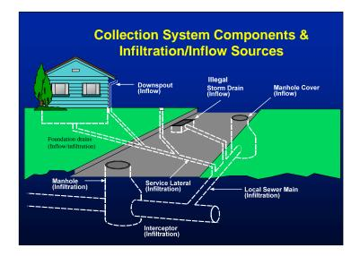
Figure D-2: Pathways of infiltration and inflow into sanitary sewer systems. (Courtesy of EPA Publication: Computer Tools for Sanitary Sewer System Capacity Analysis and Planning, EPA/600/R-07/111).
