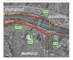
ALCOSAN is evaluating the installation of a tunnel as a regional based alternative. One of the tunnel scenarios beina evaluated would extend a tunnel to the A-42 CSO located near Washington Boulevard in Pittsburgh. This CSO is the largest (by volume) in the ALCOSAN service area. large Addressing this overflow will be an important component of the Upper Allegheny Basin's Facility Plan.
