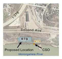
One potential control method being considered in the Main Rivers Basin is the Retention Treatment Basin (RTB). An RTB is a large tank designed to capture and treat combined sewage that would otherwise be released directly into one of our rivers or streams during wet weather events. RTBs treat the combined sewage using settling, screening and disinfection processes before it is discharged.
