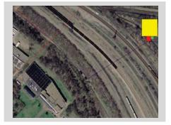
Retention Treatment Basins (RTBs) are one of the proposed technologies for the control of CSOs within the LOGR Planning Basin. The overflows from the existing CSO outfalls would be directed to these RTBs where the CSOs would be treated by screening and disinfecting the flow prior to discharge to the Ohio River. The above graphic shows a potential layout of an RTB to control the CSOs within Stowe Township.
