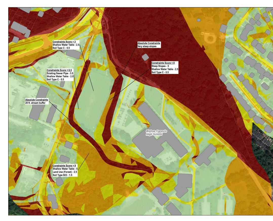
Figure 2. Example Showing the Overlay of Constraint Layers and the Resultant Scores
