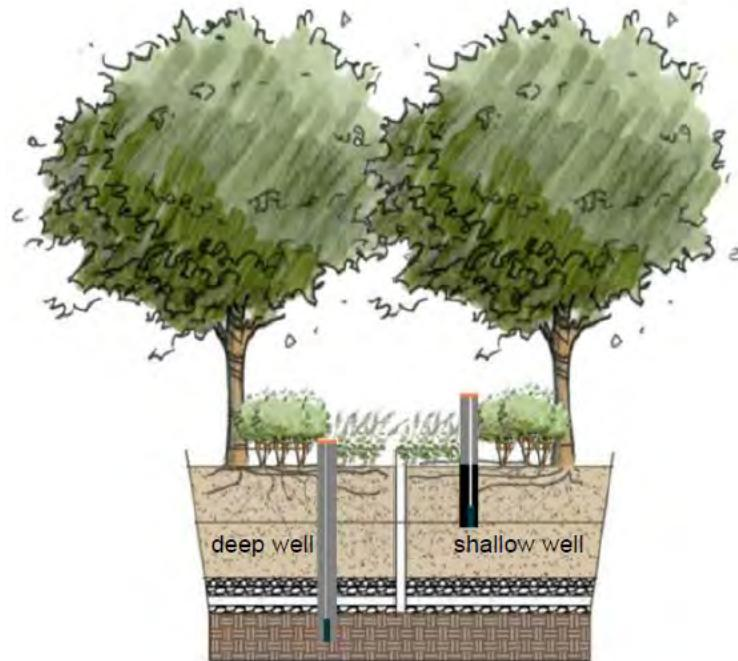
Figure 2-18. Use of a Deep Well and Shallow Well at a Bioretention Site (CVC)
