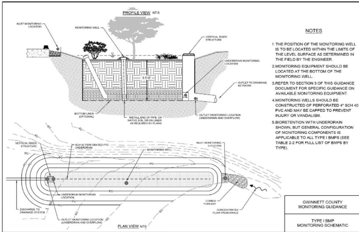
Figure 2-19. Example Schematic of a Bioretention Site (Gwinnett County)
