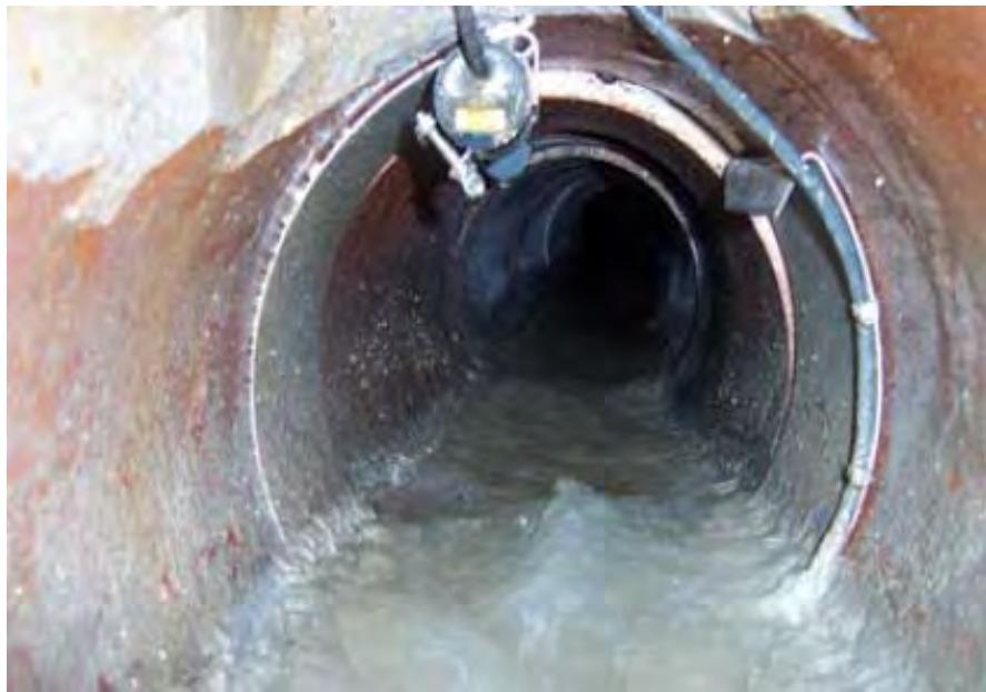
Figure 2-22. In-sewer Monitoring with Area-Velocity Flow Meter (ALCOSAN)
