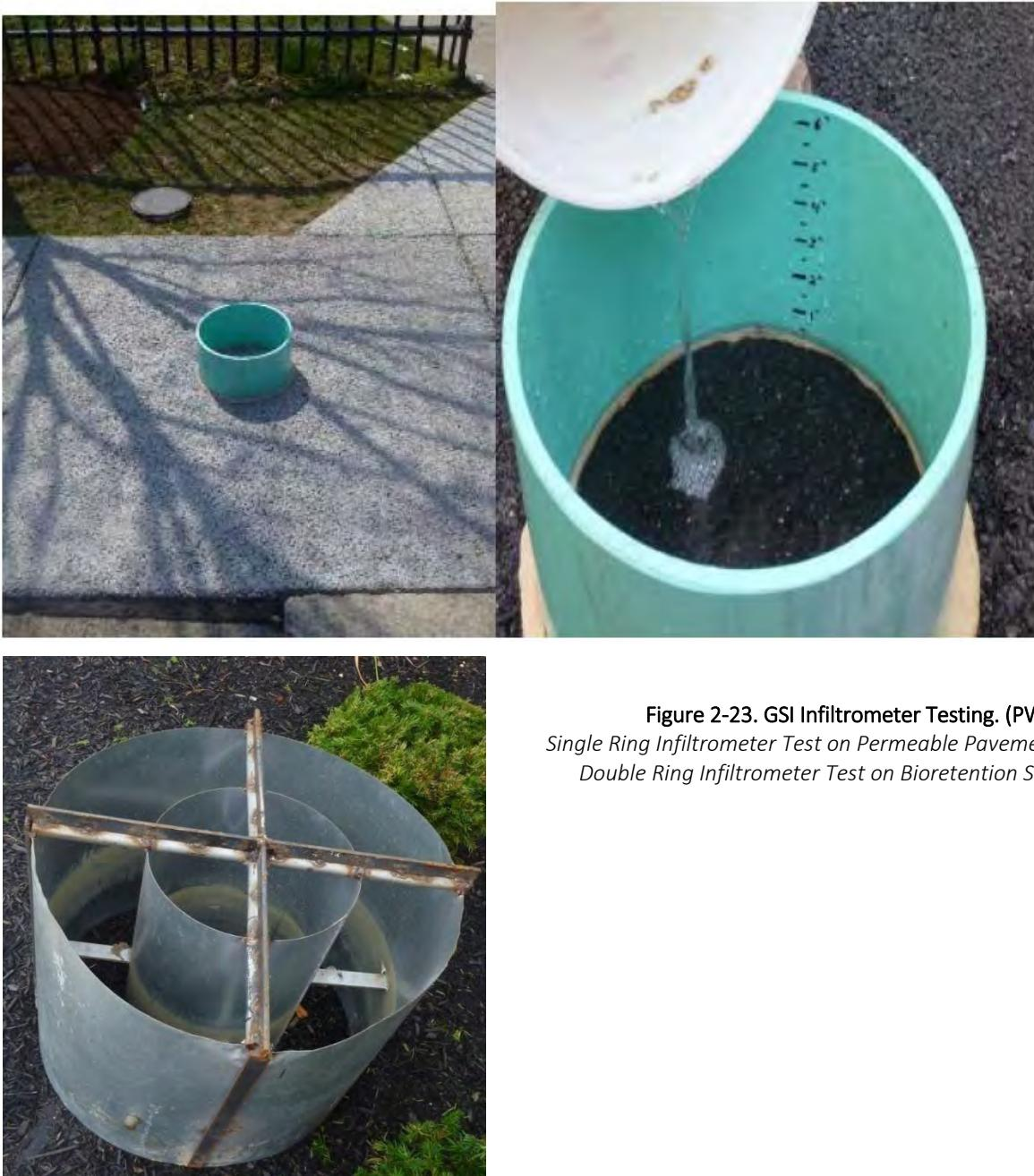
**Figure 2-23. GSI Infiltrometer Testing. (PWD)**
