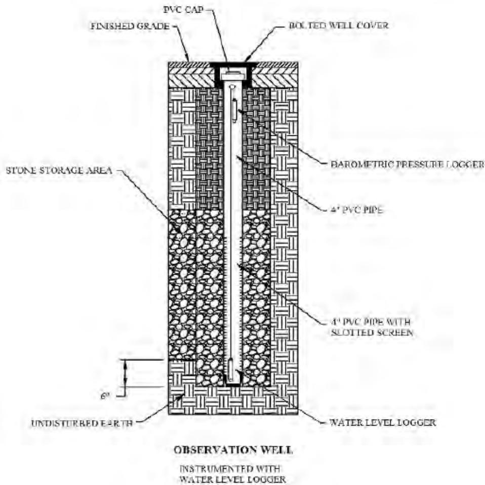
**Figure 2-17. Example Monitoring Well Schematic (PWD).**
