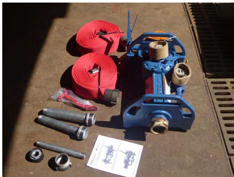
Figure 2-15. Simulated Runoff Test Equipment (PWD)
