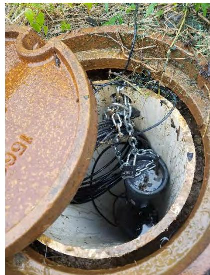
Figure 2-12. Pressure transducer installed in monitoring well (PWSA)
