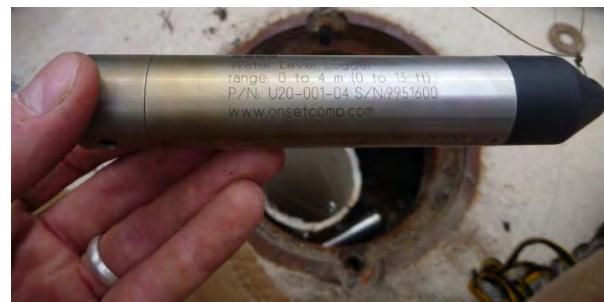
Figure 2-11. Onset HOBO Pressure Transducer (PWD)
