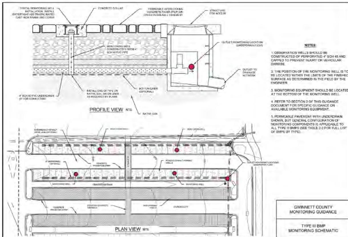
Figure 2-20. Example Schematic of a Permeable Pavement Site (Gwinnett County)
