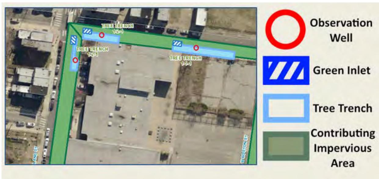
Figure 2-3. Layout of Observation Wells for in-GSI Monitoring of Three Tree Trenches (PWD)
