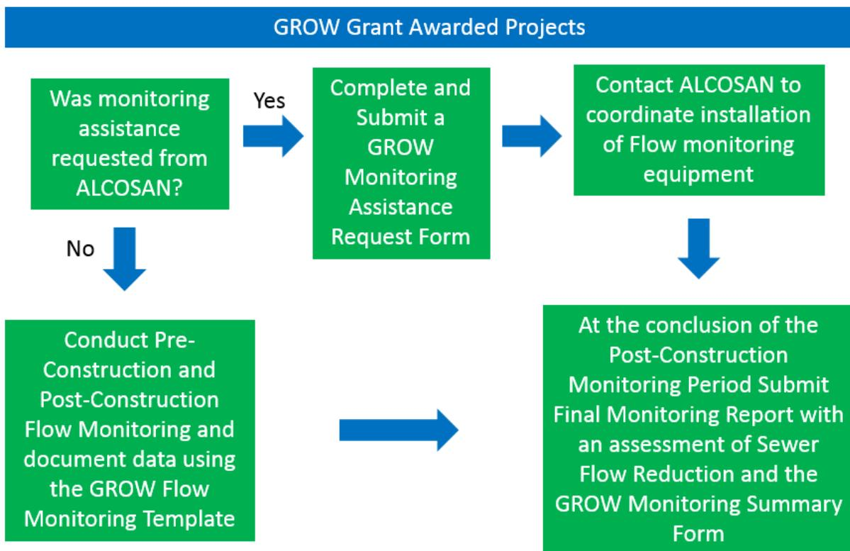
Figure 1-1. Monitoring Process Flowcharts for Pre- and Post-Construction Monitoring
