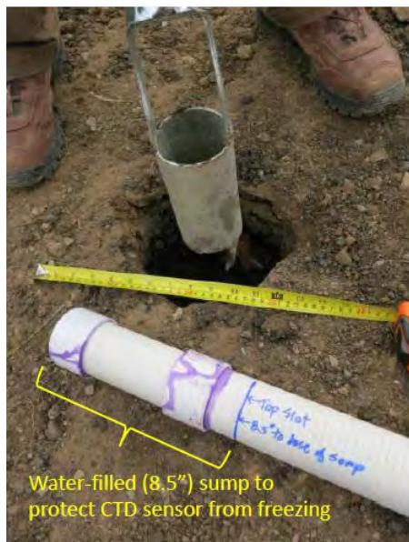
**Figure 2-24. Field measurement of sump depth**
