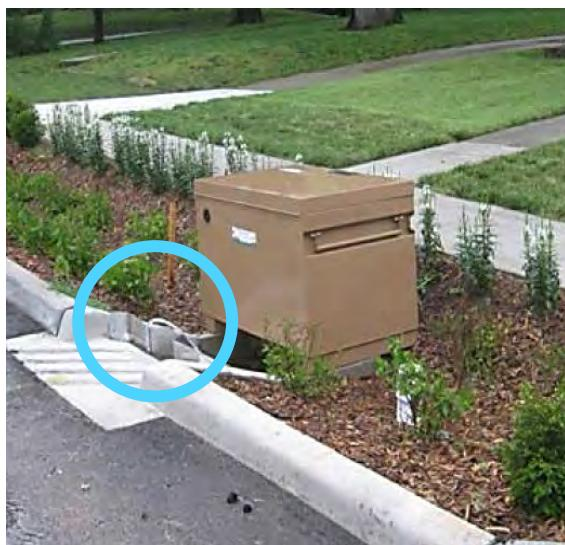
Figure 2-13. Bubbler Level Sensor Installed on Flume for Inflow Measurement (Kansas City)
