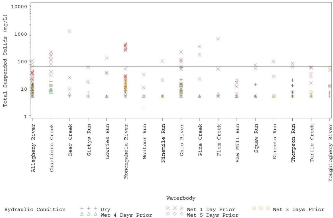
**Figure 5-25: Percent of Samples Exceeding 60 mg/L Reference Threshold**
