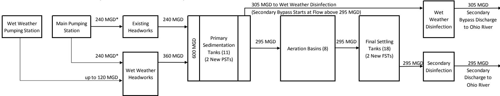
\* Flow distribution from Main Pumping Station will be optimized to provide efficient and reliable operation
