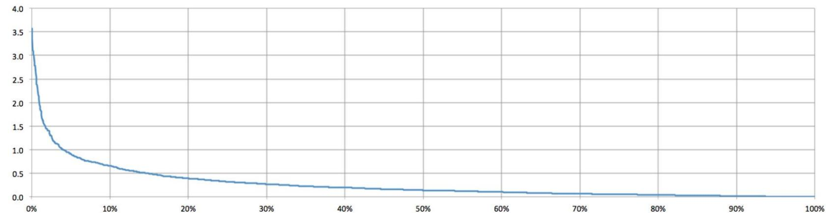
The top 12.6% highest net runoff ranked inlet locations appear to receive 50% of runoff tributary to known inlets in sheds A-22 through A-35.
