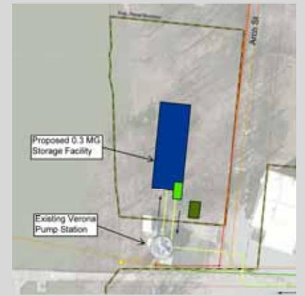
**A below grade 0.3 MG storage facility being proposed at the existing Verona Pump Station will provide control during the 2-year design storm and allow for a possible recreational use of the land above.**
