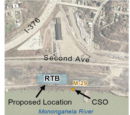
One potential control method being considered in the Main Rivers Basin is the Retention Treatment Basin (RTB). An RTB is a large tank designed to capture and treat combined sewage that would otherwise be released directly into one of our rivers or streams during wet weather events. RTBs treat the combined sewage using settling, screening and disinfection processes before it is discharged.
