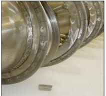
Field replaceable sintered tungsten carbide tiles the entire length of the scroll
