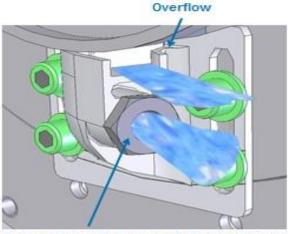
Exchangeable nozzle to control the liquid level inside the rotor more accurately, reducing the cresting.
