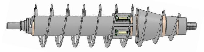
Thanks to the open flight design the centrate travels in a direct path to the discharge, flowing parallel to the length of the scroll. This is an improvement over outdated full-flight designs that forced the liquid flow to travel in a spiral path in the opposite direction of the conveyed solids.
