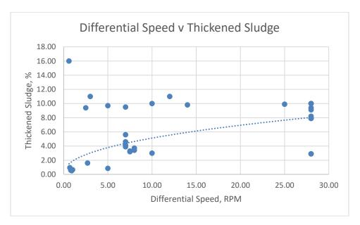
Table: 2 Bowl Speed vs Thickened Sludge (Alfa Laval)
