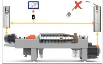
for an immediate restart once power is restored. Click on the image to see how it works
