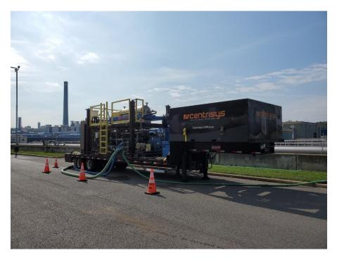
Figure 2. Trailer mounted Centrisys THK200 thickening centrifuge skid.
