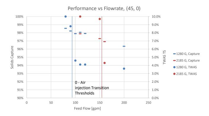
Figure 8. Impact of feed flow on performance with nozzles at (45°, 0°) at two G-levels.
