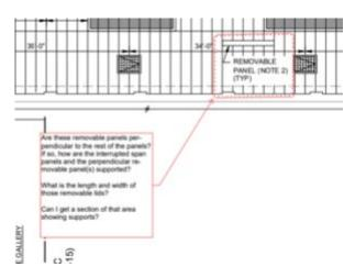
**Answer:** Intention is that removable panel is fabricated from tread plate or similar by others and will cover the area at the location of the stop plates. Panels should be supported by typical precast hangers that span the (5) adjacent panels.
