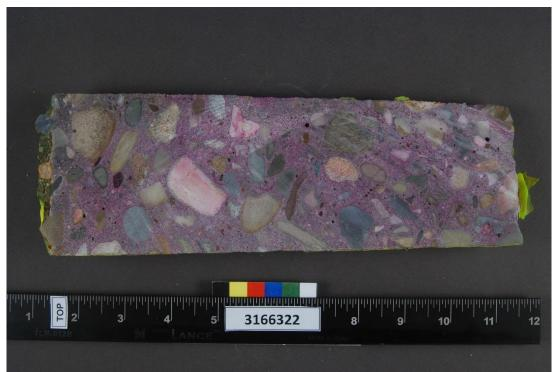
Figure 2. Lower level S-1 (3166322). Photograph of freshly cut surface with phenolphthalein indicator applied. The surface of the core was coated with fluorescent dyed epoxy before cutting.
