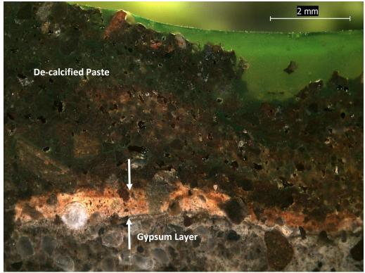
Figure 5. Lower level S-1 (3166322). Stereo-optical micrographs showing porous, de-calcified paste along the surface and a layer of gypsum desposits highlighted by the two arrows.
