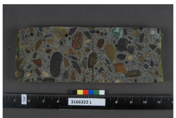
Figure 3. Lower level S-1 (3166322). Photograph of polished cross sectioned slab. The surface of the core was coated with fluorescent dyed epoxy before cutting.
