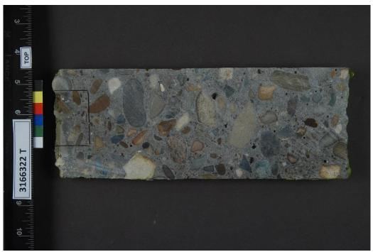
Figure 6. Lower level S-1 (3166322). Photograph of cross sectioned slab showing location of thin section preparation outlined in black.
