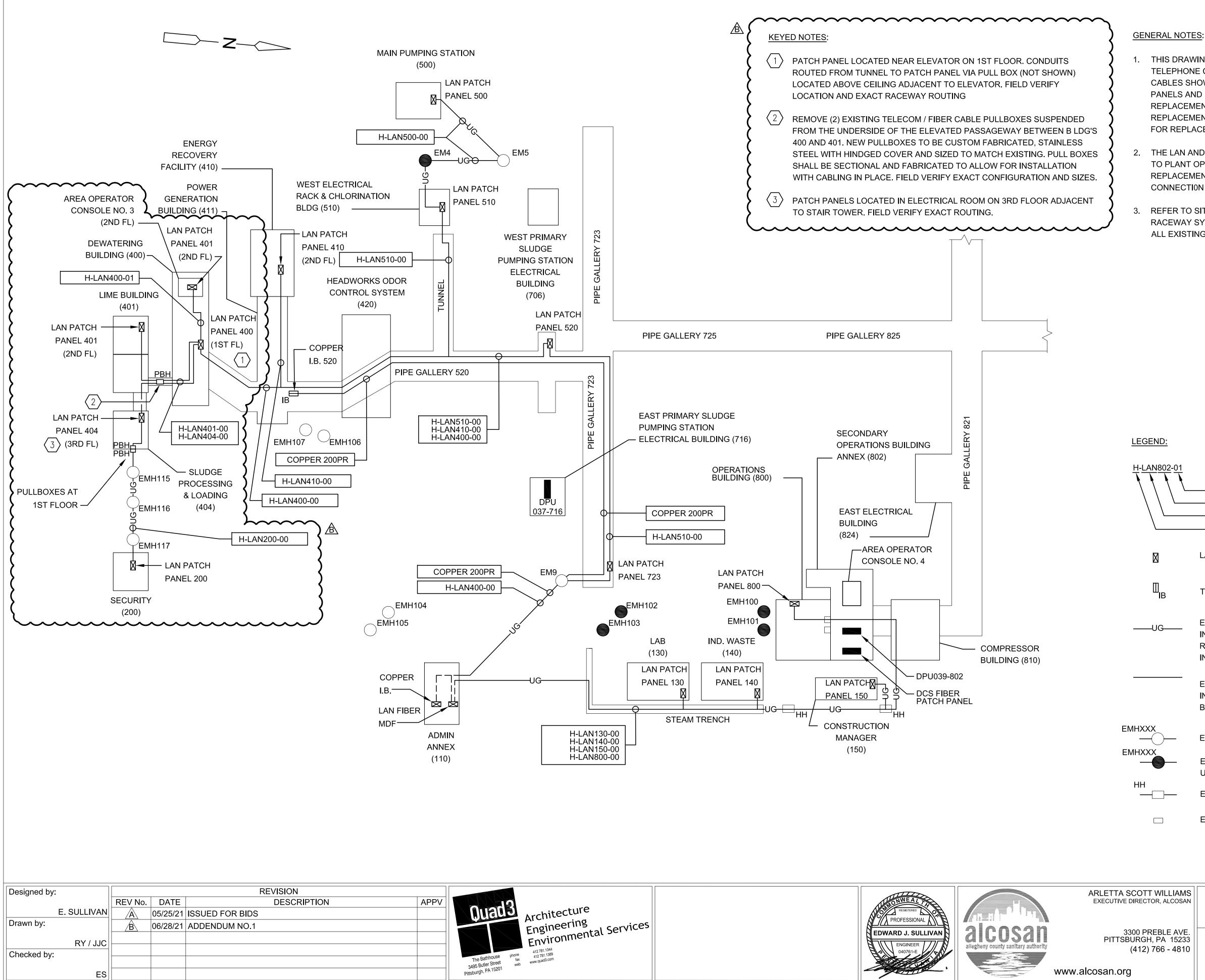
1. THIS DRAWING DEPICTS THE REQUIRED LOCAL AREA NETWORK (LAN) FIBER AND TELEPHONE COPPER CABLING REMOVALS. ALL INDICATED LAN AND TELEPHONE CABLES SHOWN ON THIS DRAWING SHALL BE REMOVED. ASSOCIATED PATCH PANELS AND INTERCONNECT BOXES (I.B.) SHALL REMAIN AND BE REUSED FOR REPLACEMENT CABLING WHERE APPLICABLE. REFER TO DWG 000-FR-01 FOR REPLACEMENT CABLE DETAILS. EXISTING RACEWAYS SHALL REMAIN AND REUSED FOR REPLACEMENT FIBER WHERE INDICATED.
