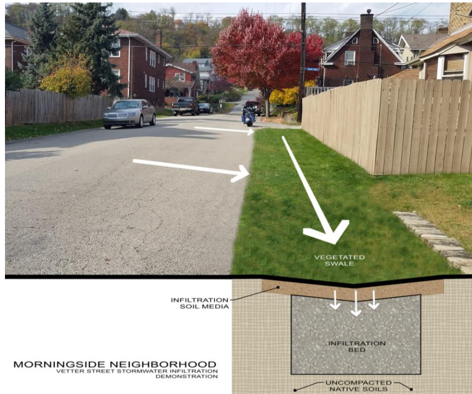
Figure 10-58: Morningside Infiltration Trench Rendering
