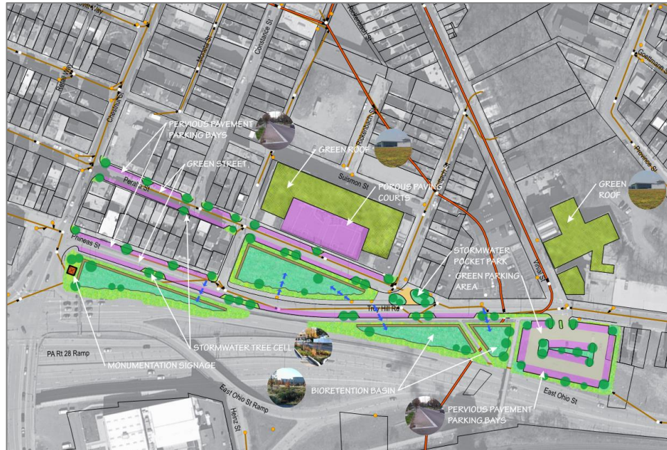
Figure 10-40: Spring Garden Green Stormwater Infrastructure Concept Design
