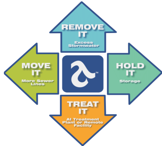
Figure 10-1: Four Categories of Sewer Overflow Control Technologies
