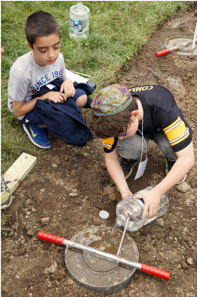
Students of ALCOSAN's annual Summer Science camp use a double-ring infiltrometer to measure the infiltration rate of soil in a planned rain garden.
